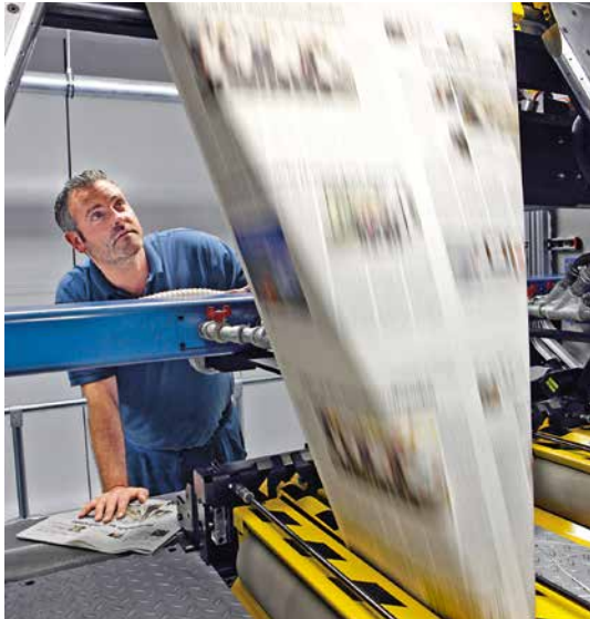
Left: Cortina press line with dryer for heatset production without ink changes at the Eco Print Center of media house De Persgroep in Belgium
